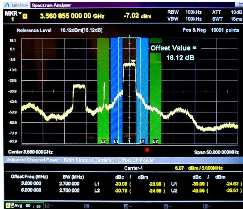
Figure 4.7: Output Spectrum of RENEW. The RENEW PA is set to an output power of 6 dB. The ACLR is -31 dBc on each of the first adjacent channels. The true BB center frequency is seen as the impulse, and an image is present opposite of the center frequency.
