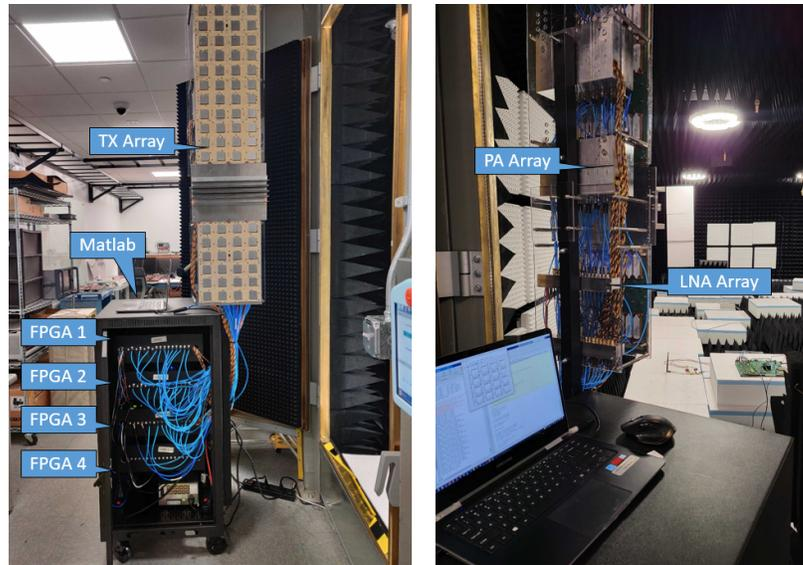
Figure 4.1: Photos of the MIMO PA Testbed.
